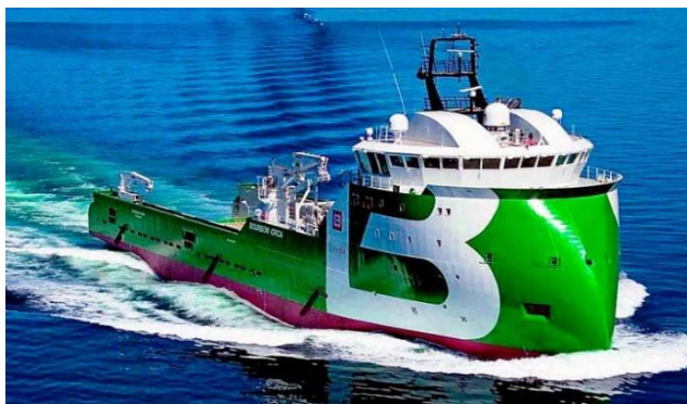
Fig. 1. Ship "Bourbon Orca" with technology X-BOW, 2006
